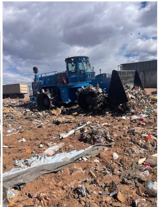
Sandoval County Landfill Compactor at Work
